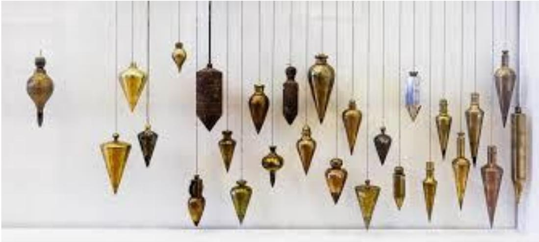
The plummet is more accurate a measuring tool than any other leveling device available, including the fancy laser levels we nerd out over, and it is the perfect metaphor for this situation. A plumb bob ***never*** lies. It always settles and aligns at the bottom to precisely the same location that it is at the top of a thing. That's the meaning of plumb – the bottom and top of a thing are aligned vertically. A plumb line helps you find that perfect alignment when you use it to measure.
